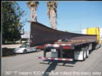
36" I beam 100' radius rolled the easy way
